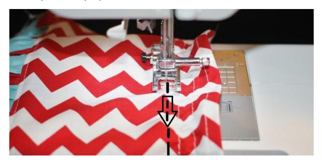
Sew all the way to the sides and when you turn directions to start a new row, give the elastic thread a little bit of slack. Finish your last row close to where the skirt part begins and not farther apart than 1/2". This is now your completed shirred bodice:
